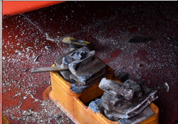
Figure 16: Broken turnbuckle (Source: German Waterway Police)
