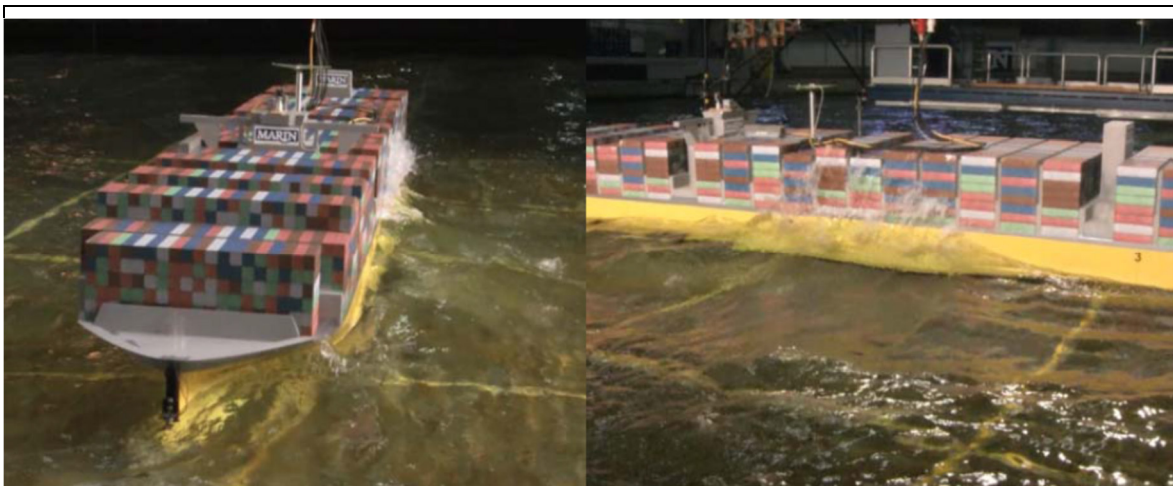
Figure 52: Images of the ship model and green water effects (source MARIN).
