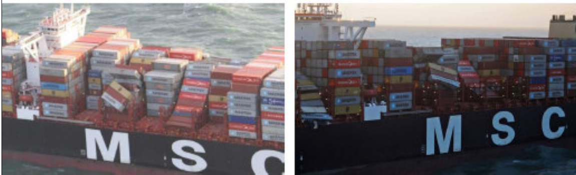
Figure 4-41: Loss of containers on the wave (port) side of the MSC Zoe, in the area where during the model tests the largest number of green water events was observed (view for port side).
